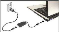
Figure 1 - 2 - Computer with AC/DC Adapter Plugged-In
